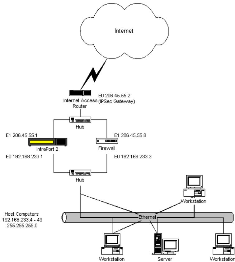
IP Static Route = 192.168.233.3 This points at the firewall or proxy that will connect VPN traffic with the Internet.
