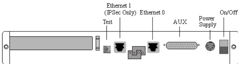
Figure 1. IntraPort 2/2+ VPN Access Server Back Panel
