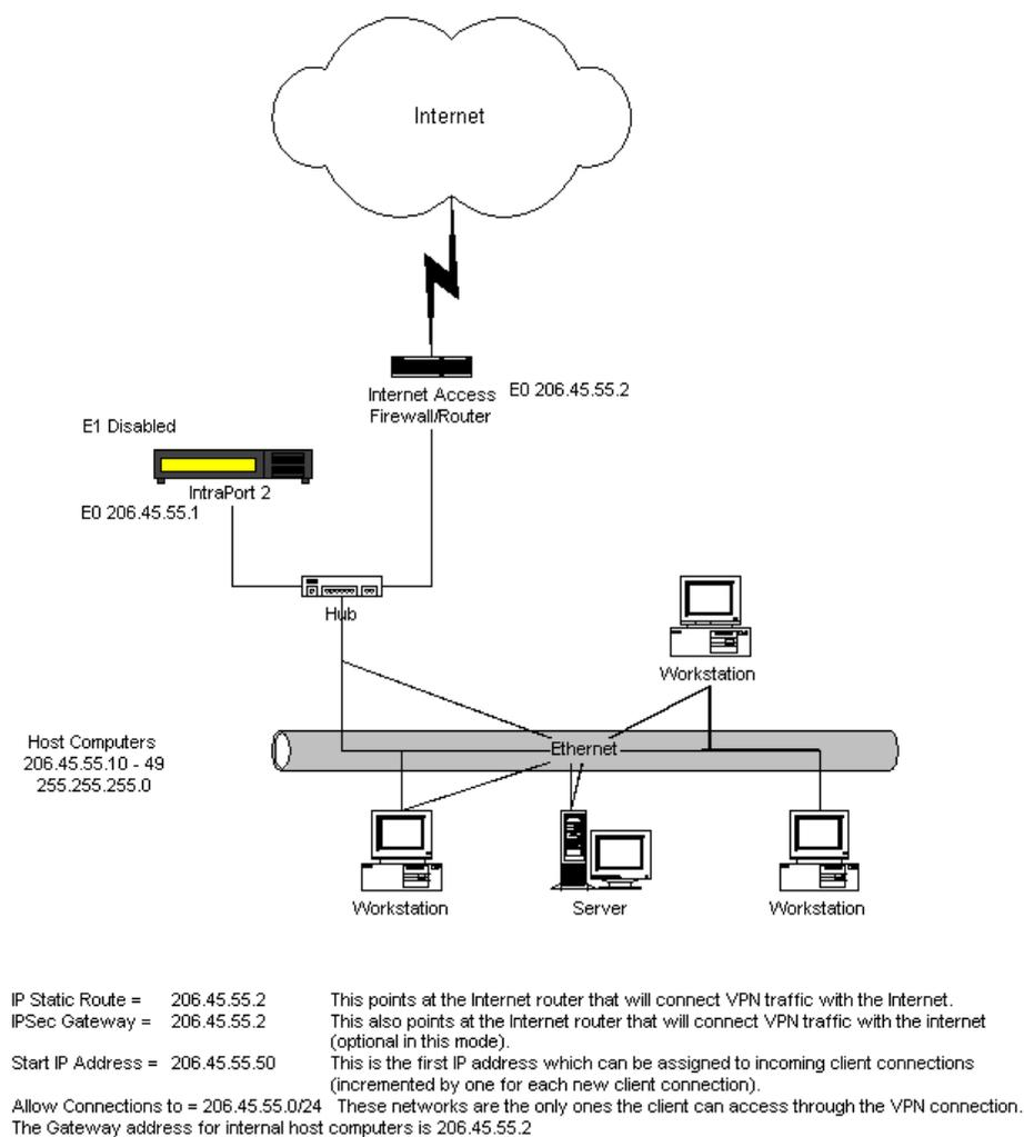
Figure 3. Diagram of Single Ethernet Setup
